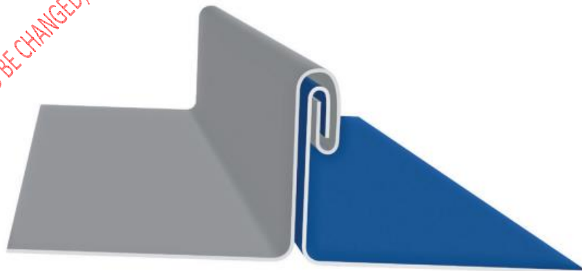
LAP DETAIL (180 DEG, MECHANICAL SEAM)
