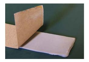
BUTYL TAPE-SEAL™ is made from a blend of elastomers, butyl, EPDM rubber, and proprietary co-polymers.
